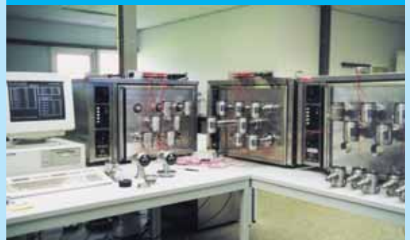
Active temperature compensation of all transmitters.
