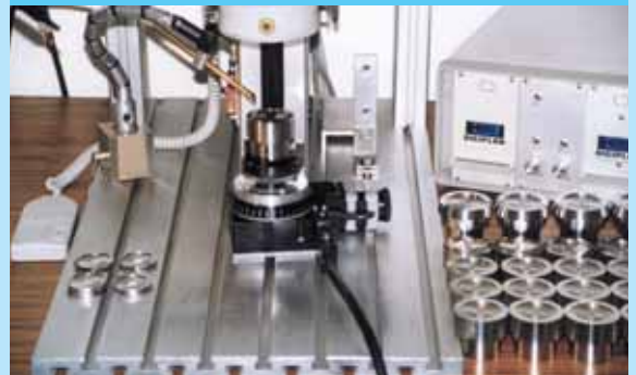
Laser welding of diaphragms.
